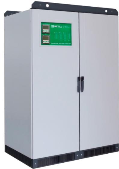
The instrumentation consists of two multi-task digital line analyzers which are able to provide with information regarding the status of the lines upstream and downstream the voltage stabilizer (phase and linked voltages, current, power factor, active power, apparent power, reactive power, etc.)
